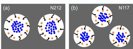
Small angle scattering experiments have shown the radius of water channels in N117 is smaller than that in N212<sup>[3]</sup>.
