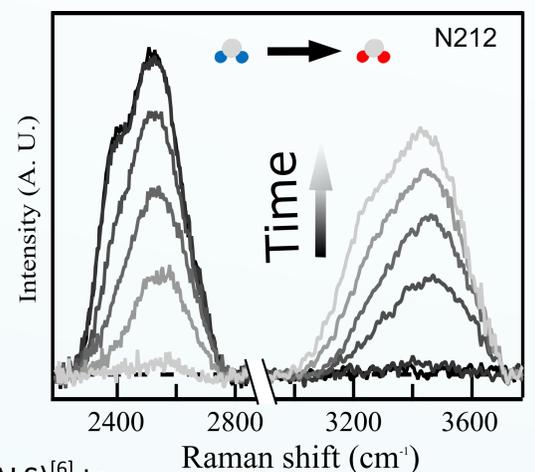
Multivariate Curve Resolution-Alternating Least Square (MCR-ALS)<sup>[6]</sup> to resolve the spectral signature of water species (H<sub>2</sub>O, D<sub>2</sub>O, HOD).
